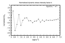
There is an oscillatory behaviour as the initial crack length increases, but it tends to  $k_{1 \text{ static}}$ .
