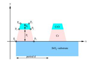
$$h_i := p_i, i = 1, 4, \quad h_i := \frac{p_i}{period}, i = 2, 5, 7, \quad h_i := \frac{p_i}{p_{i-1}}, i = 3, 6, 8$$
