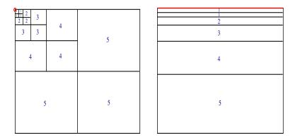
meshes graded toward singular points or towards interfaces h-p methods: variable polynomial degree of FE function adaptive mesh generator controlled by local error estimator
