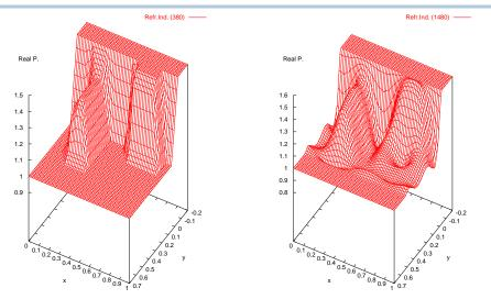
given and reconstructed refractive index over cross section of grating
