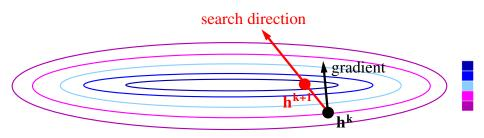
gradient computation: search direction for new iterate  $h^{k+1}$ line search for new iterate new computations for objective functional required
