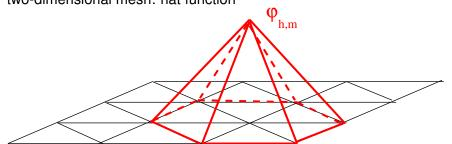
For Helmholtz equation, piecewise linear nodal basis over hexagonal two-dimensional mesh: hat function  $\phi_{h,m}$
