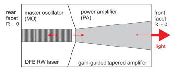
Fig. 1. Top view of a MOPA device consisting of a DFB Master Oscillator (MO) and a tapered Power Amplifier (PA).
