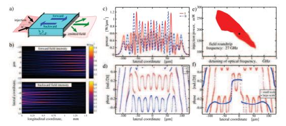
Fig. 1 Evidences of spatial rocking in broad emission area semiconductor lasers: (a): the scheme; (b): the characteristic spatial field intensity distributions, representing one of two phase-locked states; (c): intensities and (d): phases of two different stable space patterns (near fields) due to the spatial rocking; (e): parameter domain of coexisting stable phase locked states. Black square indicates parameters used in panels (b-d); (f): phase soliton.
