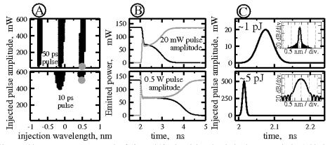
Fig. 2. Upper and lower rows represent a study of 50ps and 10ps long injected optical pulses, respectively. A: black areas show wavelengths and amplitudes of the injected pulses realizing the switching between two states. B: time traces during the state switching. C: resonant injected CW pulses corresponding to the grey dots in panel A and implying the switching between two states shown in panel B. Inserts: optical spectra of these pulses. Dotted lines: SRL resonances.
