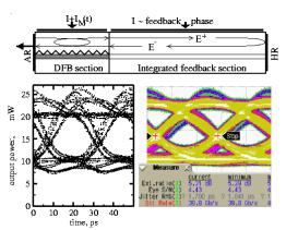
**Fig. 1** Top: scheme of a PFL, consisting of an antireflection coated DFB- and high-reflection coated IFB sections. Bottom: eye diagrams of simulated (left) and measured (right) response of the PFL to a PRBS current modulation (NRZ).
