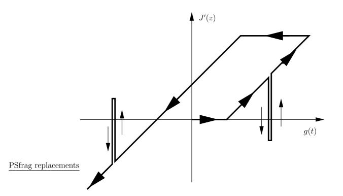
Figure 1: Stress-strain diagram for the model in Example 4.7: Horizontal lines correspond to sticking  $(\hat{z} = 0)$ , lines parallel to the diagonal correspond to motion under dry friction  $(0 < |\hat{z}| < 1)$ , and vertical lines correspond to viscously slipping motions  $(|\hat{t}| = 0)$ .
