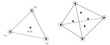
Fig. 5.8 The cubic Hermite element.
