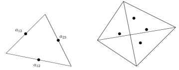
**Fig. 5.9** The finite element  $P_1^{\text{nc}}(K)$ .
