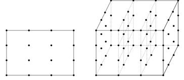
**Fig. 5.12** The finite element  $Q_3(K)$ .
