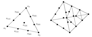
**Fig. 5.7** The finite element  $P_3(K)$ .
