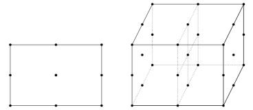
**Fig. 5.11** The finite element  $Q_2(K)$ .
