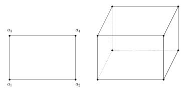
**Fig. 5.10** The finite element  $Q_1(K)$ .
