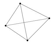
**Fig. 5.5** The finite element  $P_1(K)$ .
