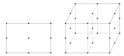
Figure 5.11: The finite element  $Q_2$ .
