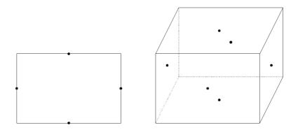
Figure 5.13: The finite element  $Q_1^{\text{rot}}$ .
