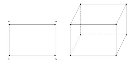
Figure 5.10: The finite element  $Q_1$ .
