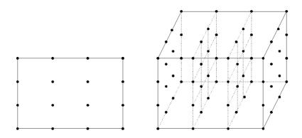
Figure 5.12: The finite element  $Q_3$ .
