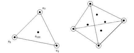
Figure 5.8: The cubic Hermite element.
