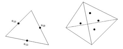
Figure 5.9: The finite element  $P_1^{\rm nc}$ .
