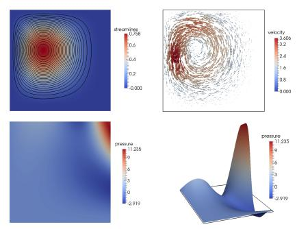
Fig. 3.1 Example 3.26. Stream function (top left) velocity (top right) and pressure (bottom). These plots are based on results obtained with numerical simulations.
