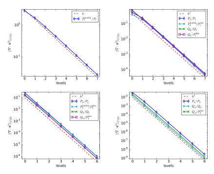
**Fig. 3.4** Example 3.27. Convergence of the errors  $\|\nabla \cdot \boldsymbol{u}^h\|_{L^2(\Omega)}$  for different discretizations with different orders k. In the top right and bottom left pictures, the magenta line is on top of the green line.
