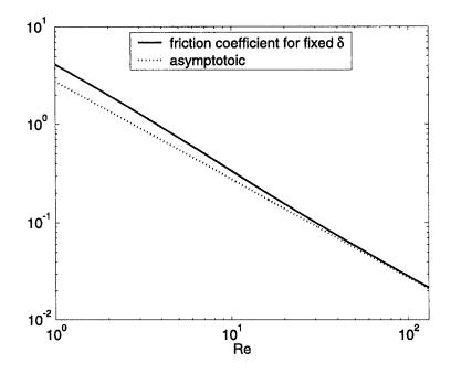
(b). Behavior of  $\beta(\delta, \text{Re})$  with respect to Re for constant  $\delta(=1)$ ,  $\gamma = 6$ ,  $V_0 = -1$ .
