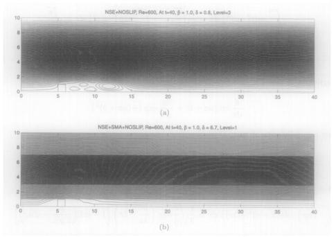
Figure 8. Two-dimensional channel with a step, the streamlines of the solution for NSE + NOSLIP on the finest mesh (a) and NSE + SMA + NOSLIP on the coarsest mesh (b) at time t = 40, Re = 600.
