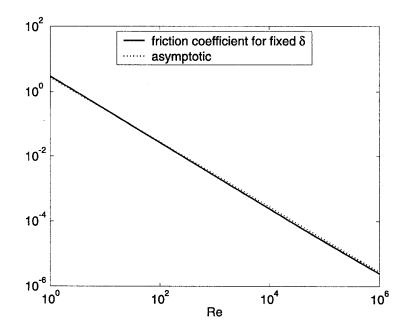
(b). Behavior of  $\beta(\delta, \text{Re})$  with respect of Re for constant  $\delta(=1)$ ,  $c_{\eta} = 1$ ,  $\gamma = 6$ . Figure 3.  $1/7^{\text{th}}$  power law boundary layer.
