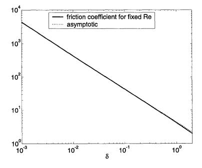
(a). Behavior of  $\beta(\delta, \text{Re})$  with respect to  $\delta$  for constant Re(=1),  $\gamma = 6$ ,  $V_0 = -1$ .
