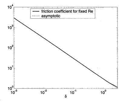
(a). Behavior of  $\beta(\delta, \text{Re})$  with respect to  $\delta$  for constant Re(=1),  $\tilde{\eta}(=1)$ ,  $\gamma = 6$ .
