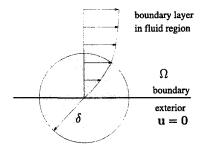
Figure 1. Averaging the velocity at the boundary does not give homogeneous Dirichlet conditions.
