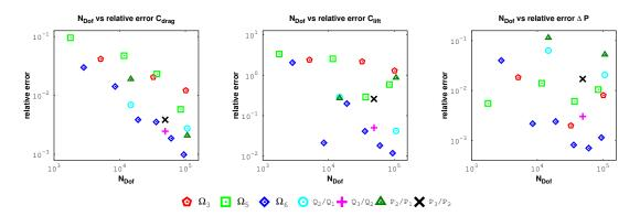
Fig. 6. Results for the three-dimensional flow around a cylinder for the IGA with third order velocity and second order pressure and for the finite element pairs  $Q_2/Q_1$ ,  $Q_3/Q_2$ ,  $P_2/P_1$ , and  $P_3/P_2$ .
