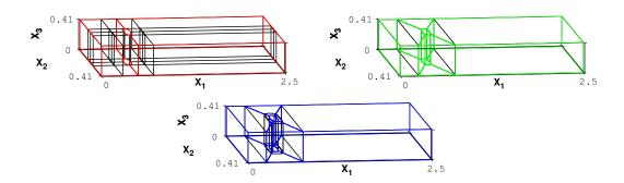
Fig. 5. Three-dimensional flow around a cylinder: Parametrizations of  $\Omega$  into patches:  $\Omega_3$ ,  $\Omega_5$ , and  $\Omega_6$ .
