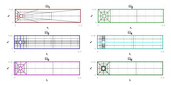
Fig. 2. Two-dimensional flow around a cylinder: Parametrizations of  $\Omega$  into patches:  $\Omega_1, \ldots, \Omega_6$ , left to right, top to bottom. The thick colored lines give the decomposition into patches, the thin lines the corresponding coarsest grids, and the dots the quadrature points. Note that  $\Omega_6$  is more refined at the cylinder than  $\Omega_2$ .
