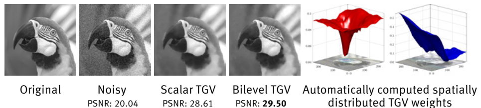
Fig. 2: Improved TGV-based denoising with automatically computed spatially distributed regularization parameters via bilevel minimization
