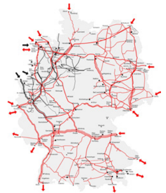
Fig. 2: German H-gas and L-gas network system of the German network operator OGE (Open Grid Europe)
