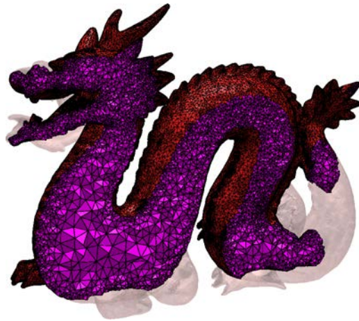
Fig. 1: Tetrahedralization of a dragon, computed with TetGen
