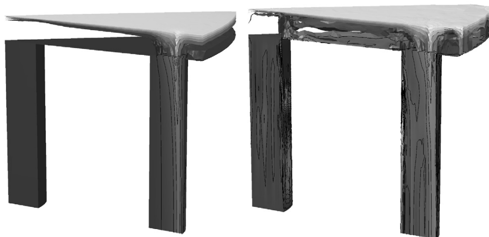
Fig. 1: H_2 concentration in the cell is bounded by its value at the inlet when using the Scott–Vogelius element for the fluid flow. Right: H_2 concentration in the cell exceeds its value at the inlet when using the Taylor–Hood element.
