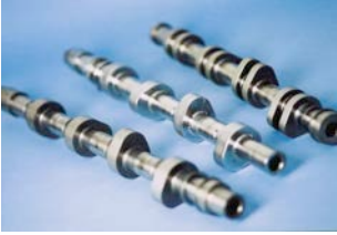
Fig. 1: Partial electron beam hardening of camshafts (pro-beam AG & Co.KGaA)
