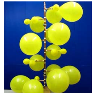
Fig. 2: Interconnected balloons exhibit two coexisting phases consisting of balloons with large (respectively, small) filling
