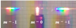
Fig. 1: A light bulb of a flashlight seen through a transmission grating (taken from http://en.wikipedia.org/wiki/File:Light-bulb-grating.png )
