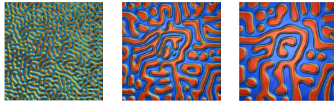
Fig. 1: Coarsening of a binary alloy: Anisotropic elasticity tensor leads to alignment of phase boundaries (Rüdiger Müller (Leibniz Group 2) and Sören Bartels (University of Bonn))
