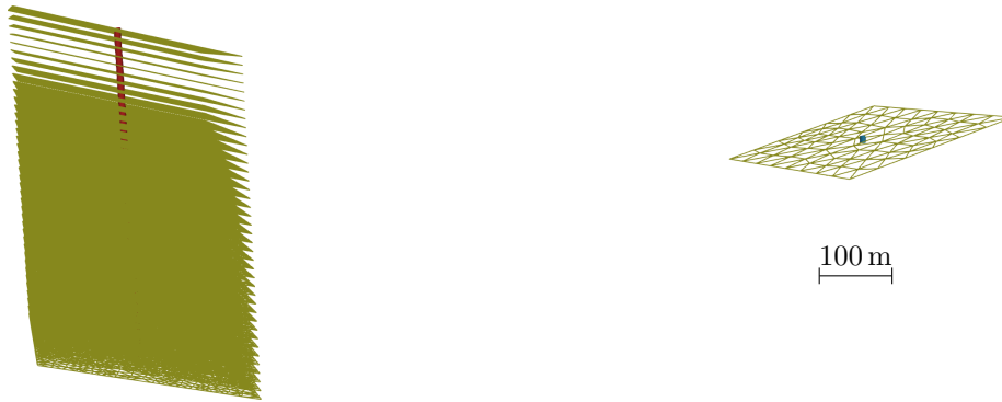
Figure 5: Alignment of the fractures and positions of the first well, w_1 (blue, on the right-hand side) and second well, w_2 (red). The olive-colored lines indicate the coarsest mesh.
