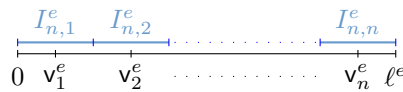
Figure 4.1: Sketch of the discretization of the edges into new vertices. Blue: Intervals I_{n,k}^e .
