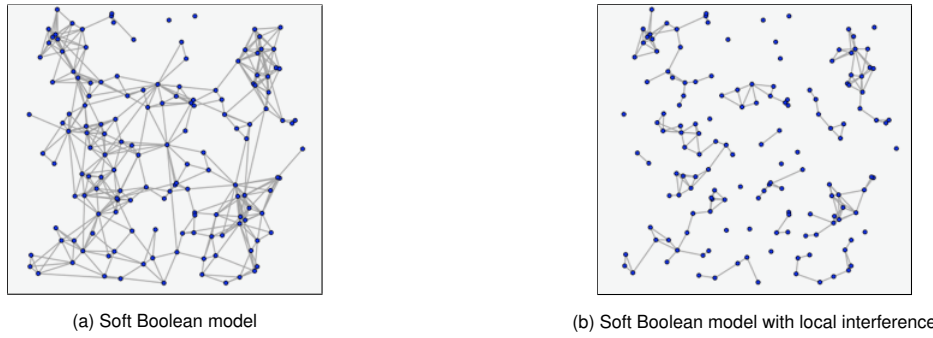
Figure 2: Examples for the soft Boolean model, Figure 2a, and the soft Boolean model with local interference, Figure 2b, on the same 150 vertices sampled from a Poisson point process of intensity \lambda = 0.04 . For the edge probabilities, the parameters \gamma = 0.65 , \delta = 2.7 , and \beta = 0.3 are used. Hence, \zeta > 0 for the soft Boolean model but \zeta < 0 for the model with local interference.
