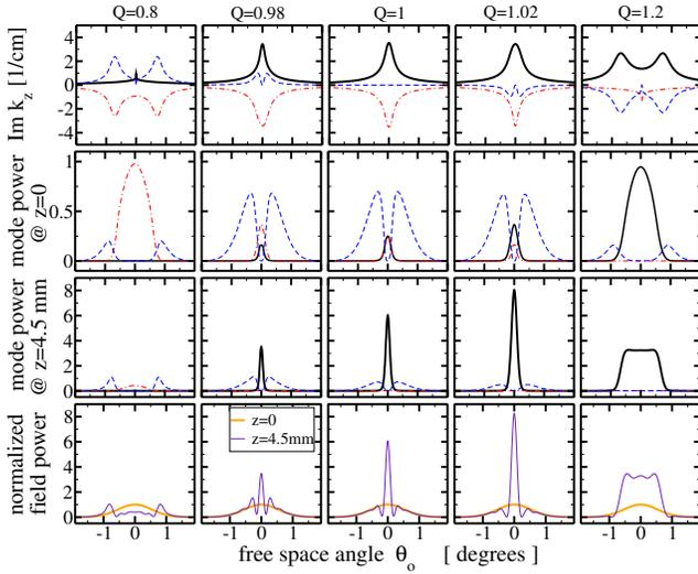
Fig. 2. Mode gain functions  $\Im m k_z$  [1st row], their contributions at  $z = 0$  [2nd row] and  $z = 4.5$  mm [3rd row], and normalized total field intensity at  $z = 0$  (thick) and  $z = 4.5$  mm (thin) [4th row] for different  $Q$  [different columns] in dependence on radiation angle.
