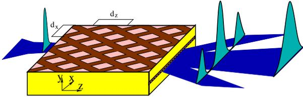
Fig. 1. Schematic representation of the periodically modulated optically injected broad area semiconductor amplifier.
