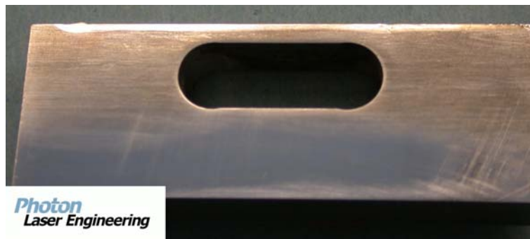
FIGURE 4. Result of a hardening experiment utilizing the computed temperature T_{hs} as set-point for the machine-based control (Courtesy of Photon Laser Engineering , Berlin, Germany).
