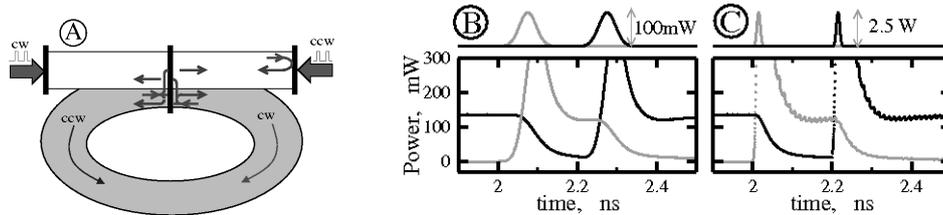
**Fig. 1** A: Scheme of an all-active SRL with indication of optical injections (thick arrows), some possible field reflections and transmissions at the coupler and at the edges of the waveguide, and directions of the CW and CCW propagating fields (thin arrows). B, C: time traces of emitted CW (grey) and CCW (black) field intensities. Top of the diagrams: a pair of consequently injected 50ps (B) and 10ps (C) long resonant CW (grey) and CCW (black) pulses implying these transitions.
