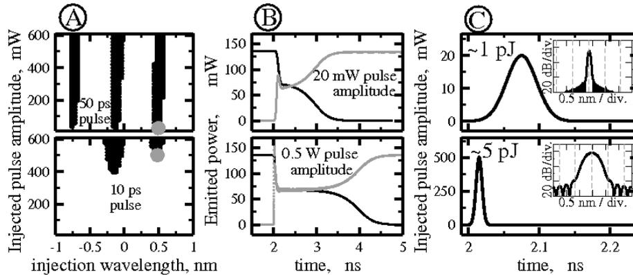
**Fig. 2** Upper and lower rows represent a study of 50ps and 10ps long injected optical pulses, respectively. A: black areas show wavelengths and amplitudes of the injected pulses realizing the switching between two states. B: time traces during the state switching. C: resonant injected CW pulses corresponding to the grey dots in panel A and implying the switching between two states shown in panel B. Inserts: optical spectra of these pulses. Dotted lines: SRL resonances.
