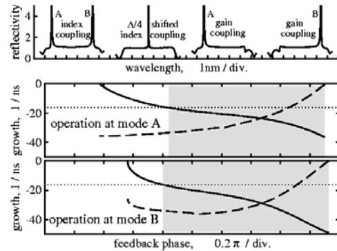
**Fig. 2** Top: reflectivity spectra of considered DFB sections. Bottom: growth (negative damping) of RO (solid) and mode interaction (dashed) resonances of the *stable* cw state in dependence on the field feedback phase. Dotted: growth of the RO resonance in solitary DFB laser. Shading: the RO damping is improved.
