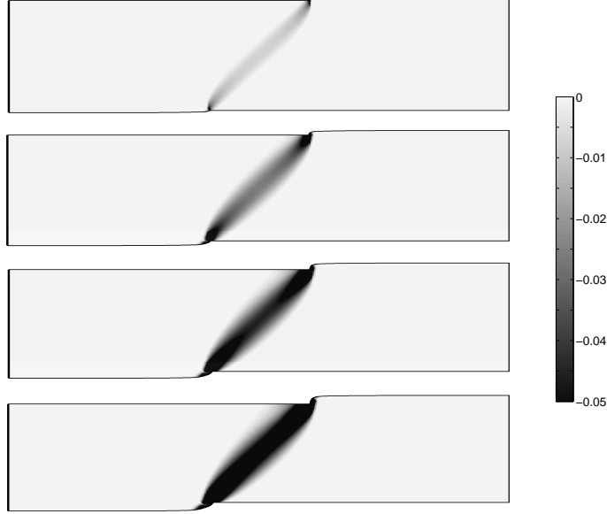
FIGURE 2. Snapshots of the time evolution of one slip-band depicted via the hardening variable \eta_h with \varepsilon = 1/64 in Example 6.1; t = 0.25\text{s} , 0.5\text{s} , 0.75\text{s} , and 1\text{s} . The displacement is magnified by a factor 4.
