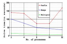
Figure 5. Solve time with a P1 element on Grid1
