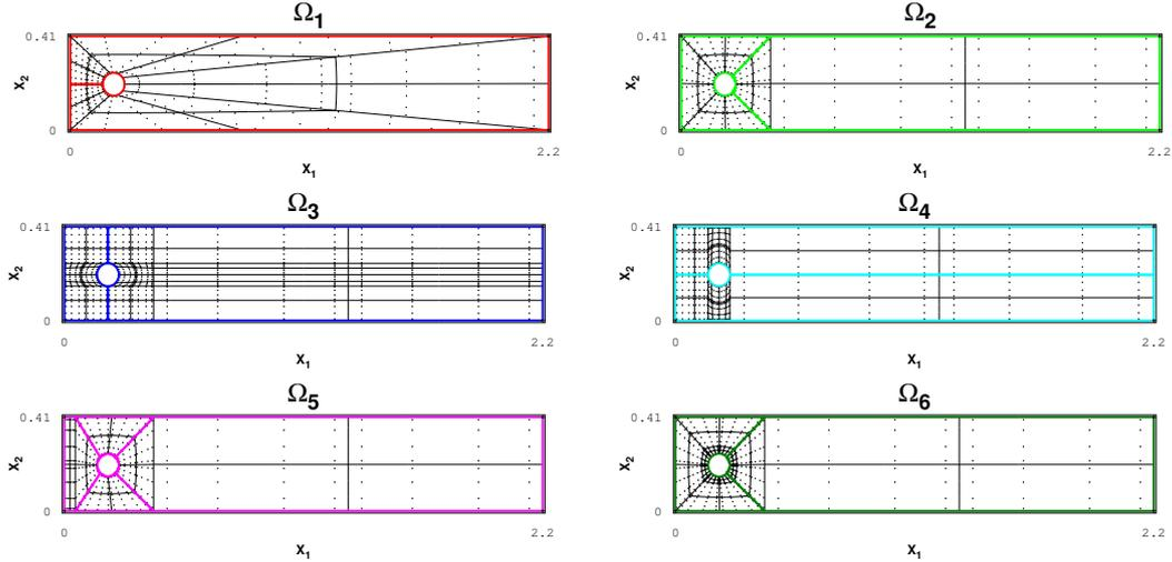
Fig. 2. Two-dimensional flow around a cylinder: Parametrizations of  $\Omega$  into patches:  $\Omega_1, \dots, \Omega_6$ , left to right, top to bottom. The thick colored lines give the decomposition into patches, the thin lines the corresponding coarsest grids, and the dots the quadrature points. Note that  $\Omega_6$  is more refined at the cylinder than  $\Omega_2$ .
