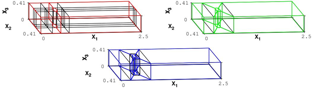
Fig. 5. Three-dimensional flow around a cylinder: Parametrizations of  $\Omega$  into patches:  $\Omega_3$ ,  $\Omega_5$ , and  $\Omega_6$ .
